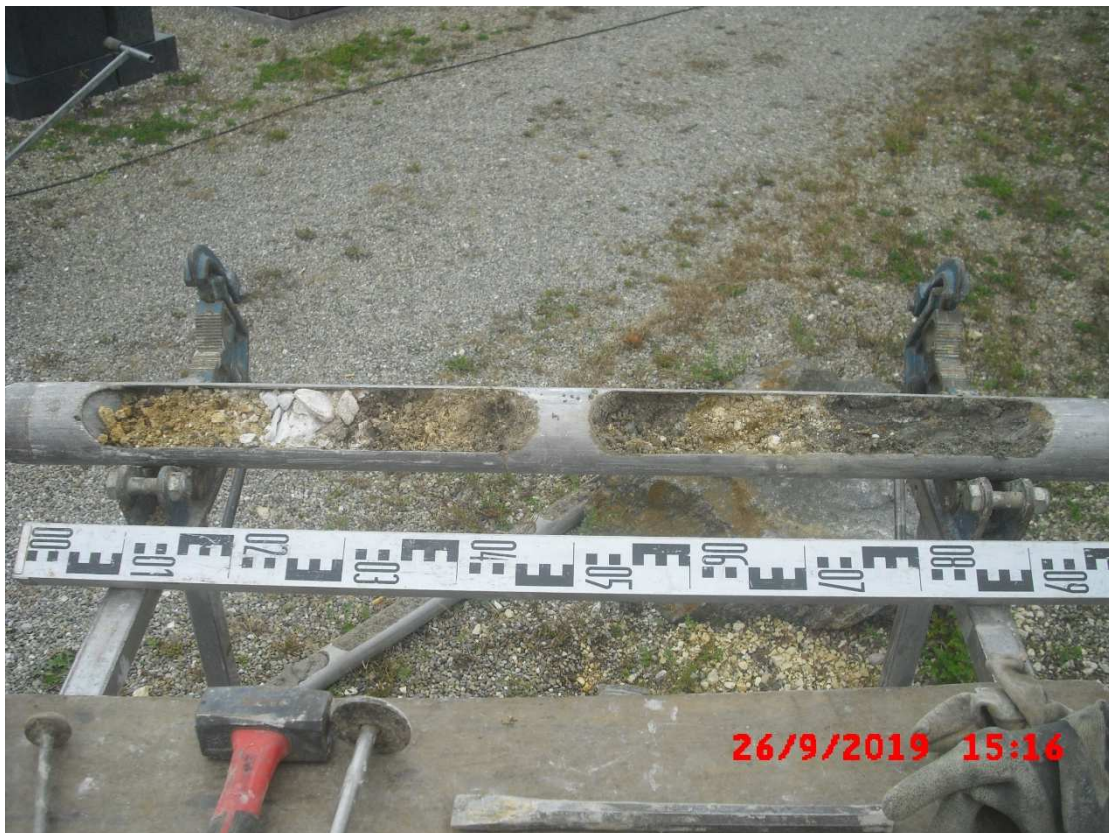
Abb. 6: Bohrkern KRB3, 0-1 m
